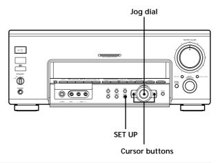
Brief descriptions of buttons and controls used to set up the speaker system
